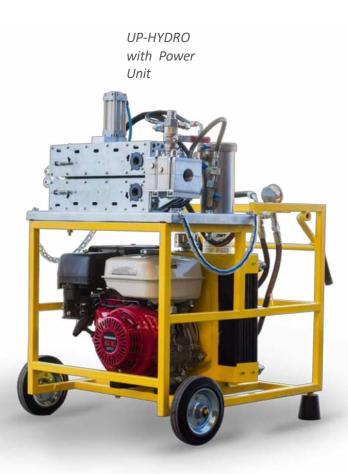
UP-HYDRO is designed to blow cable and tubes in ducts.
